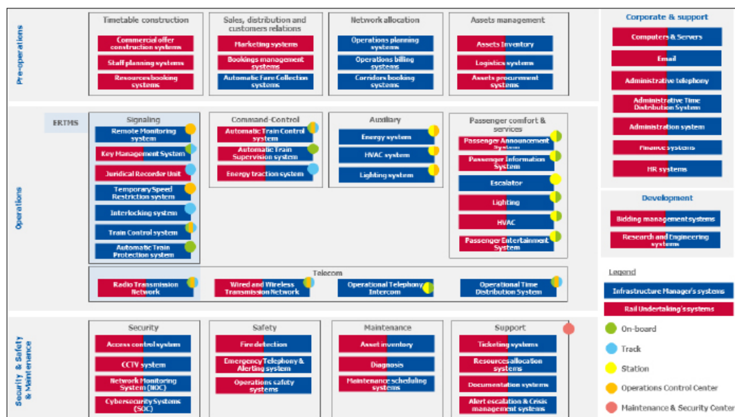
A listing of OT functions in typical railway systems (Source: ENISA Railway Security Report, 2020)
