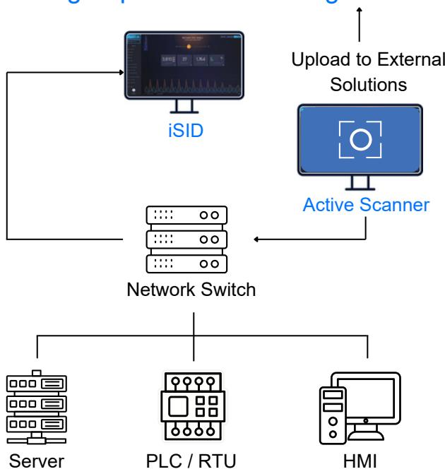
**Active Scanner** working in tandem with iSID and / or generating files for upload
