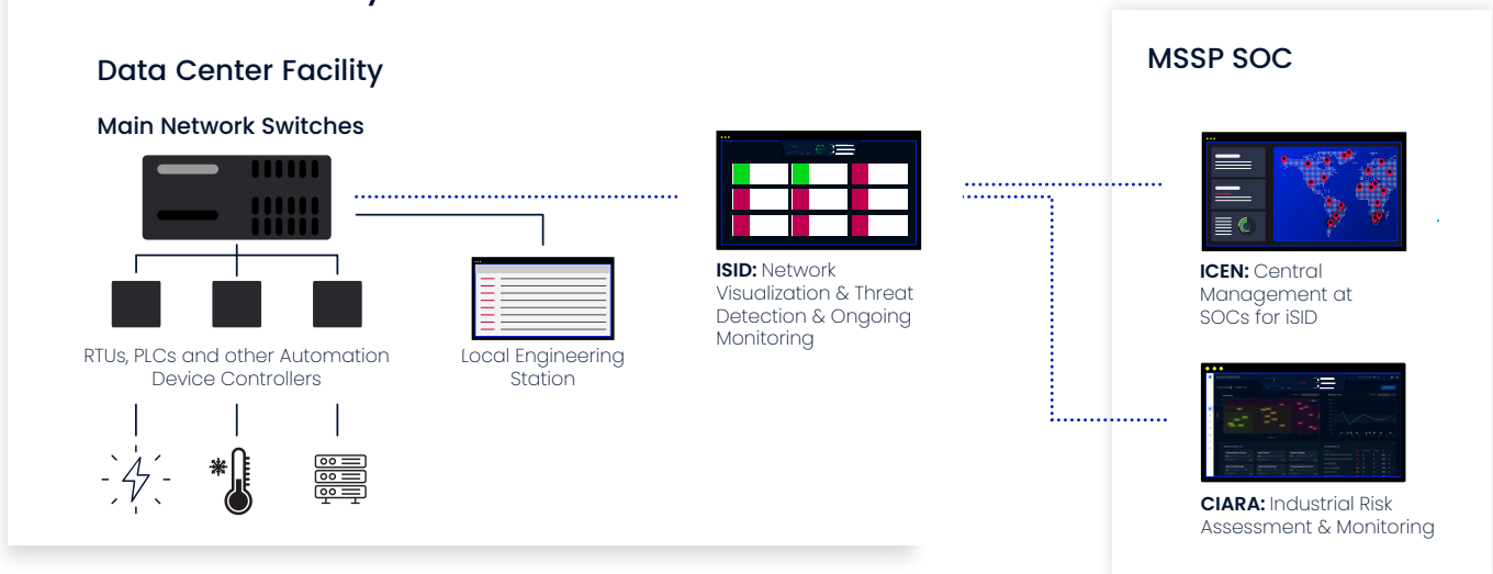
Schematic diagram of the data center project, including future threat and risk monitoring at an MSSP's SOC
